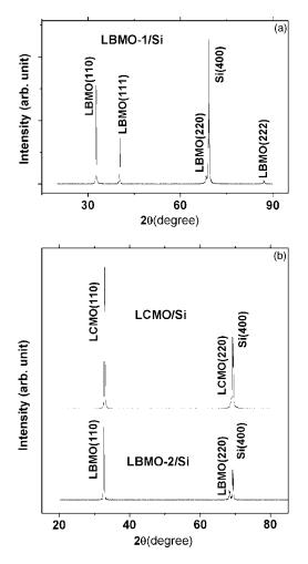
FIG. 1. X-ray diffraction spectra of (a) LBMO-1/Si, (b) LBMO-2/Si, and LCMO/Si heterojunctions.
