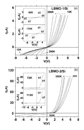
FIG. 3. Isothermal I-V curves of (a) LBMO-1/Si heterojunctions measured from 10 to 290 K with a step of 40 K and (b) LBMO-2/Si heterojunctions measured at 35, 72, 113, 160, 225, and 300 K. Insets show the response of I-V curves to magnetic field for the corresponding samples.
